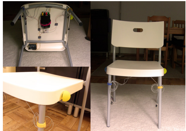
Figure 8: Final Chair with Arduino board, circuit and switches mounted.
